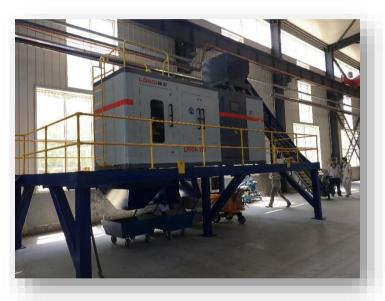
Preconcentration using XRF ore sorting technology will be used to pre- concentrate both the Merensky and UG2 ore.
